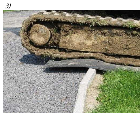
Fig. 1: Elastic deformation of a plate under heavy load
